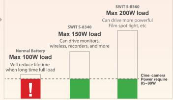
6A Charge **Fast charging** – The battery supports Max 6A charging current, halving the charging time. For example the 160Wh level battery can be charged to full within 2.5 hours, by SWIT new fast charger S-3812A/S. And the high quality contact pins ensure the reliable and safe condition under 6A current.
